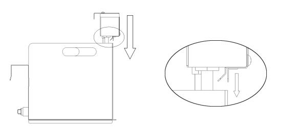
Step 1: Line up the heater module grooves with the oil vat and push down completely
