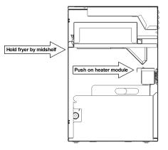
Step 3: While holding the midshelf, push on the heater module to lock it in place
